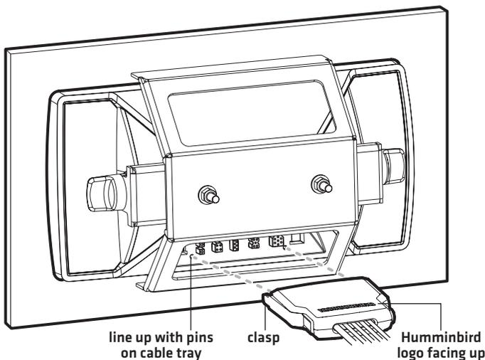
9. Pull carefully on the cable tray to confirm the installation is secure. Make sure both clasps clicked into place in step 8.
