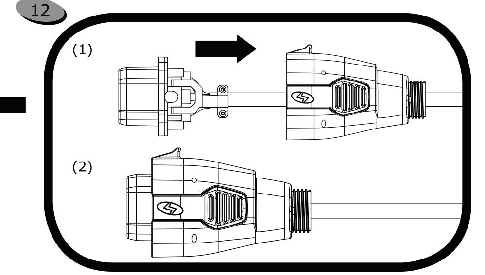
Hold cord seal and connector body in one hand as shown (1) and carefully pull cord with other hand backwards until it begins to enter connector body
