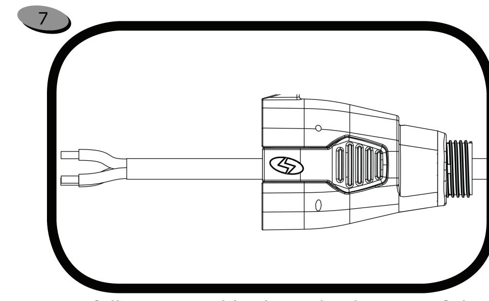
Carefully insert cable throught the rear of the connector as shown. Attempt not to fray exposed copper wire
