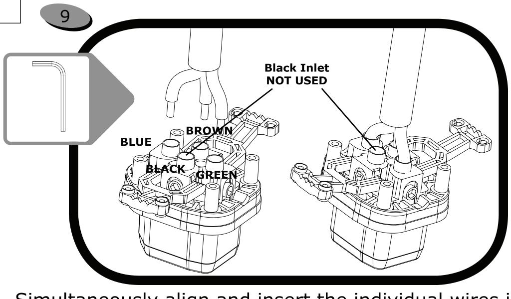
Simultaneously align and insert the individual wires into their corresponding color-coded inlets as shown. Push all wires in as far as they will go. Make sure all copper wiring is fully captured within the rear of the metal capture. Visually inspect through the clear plastic inlets that there are no stray copper strands. Use the hex key and tighten all screws to 0.1373 N-m. **Blue Inlet - Neutral Black Inlet - Not Used**
