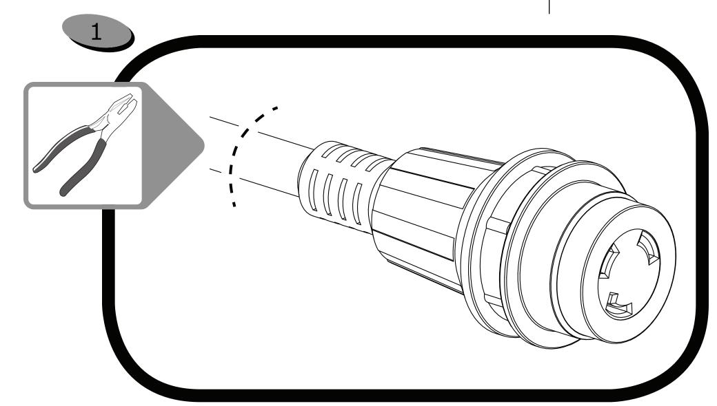
Cut female cord-end from your existing 32A/230V Cord-set. Inspect copper wires for corrosion, and cut back more cord if necessary to reach bright copper.
