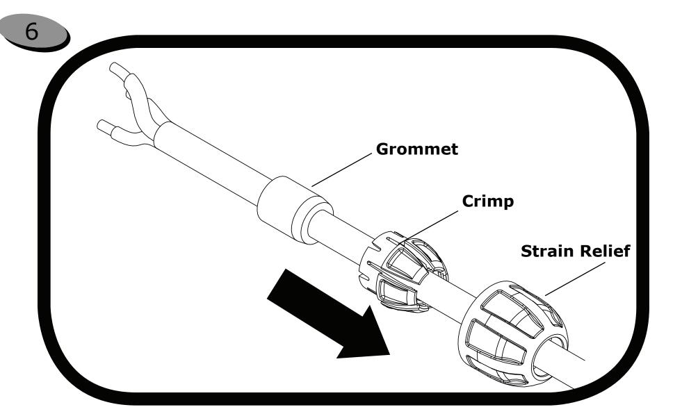
Slide strain relief, crimp and grommet onto the prepared
