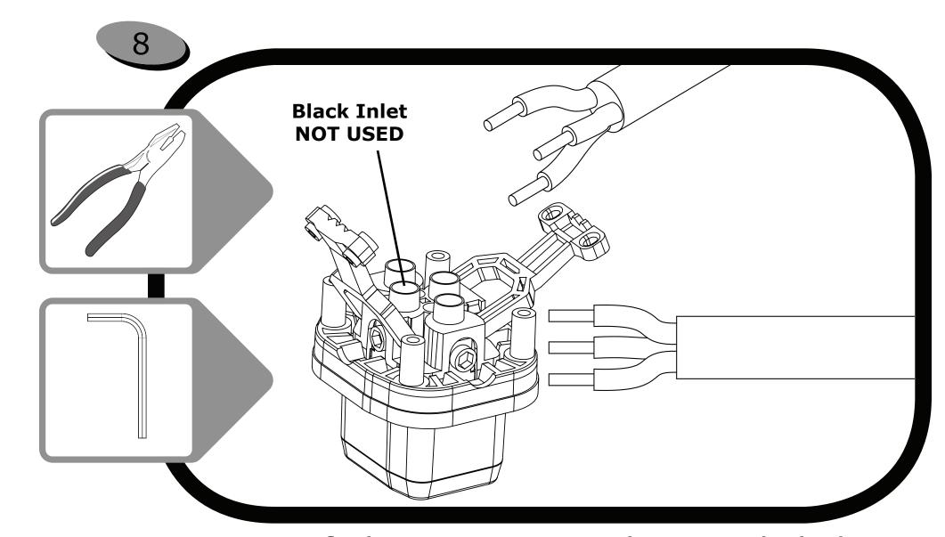
For ease of alignment, use pliers and slightly bend the ends of the conductor wires as shown. Next, use the provided hex key and loosen the set screws in the front connector assembly to allow plenty of clearance for the insertions of the copper strands into the inlet holes.
