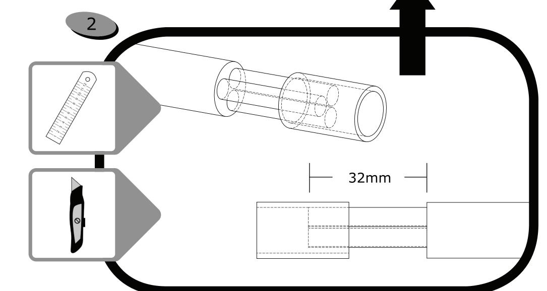
Measure 32mm back from freshly cut cord end and use marker to indicate cut. Lightly score the outer jacket with a utility knife and be sure not to cut any inner wires. Remove only the 32mm segment of outer jacket exposing the inner wires and the fibrous cord filler. Cut away all strands of filler.
