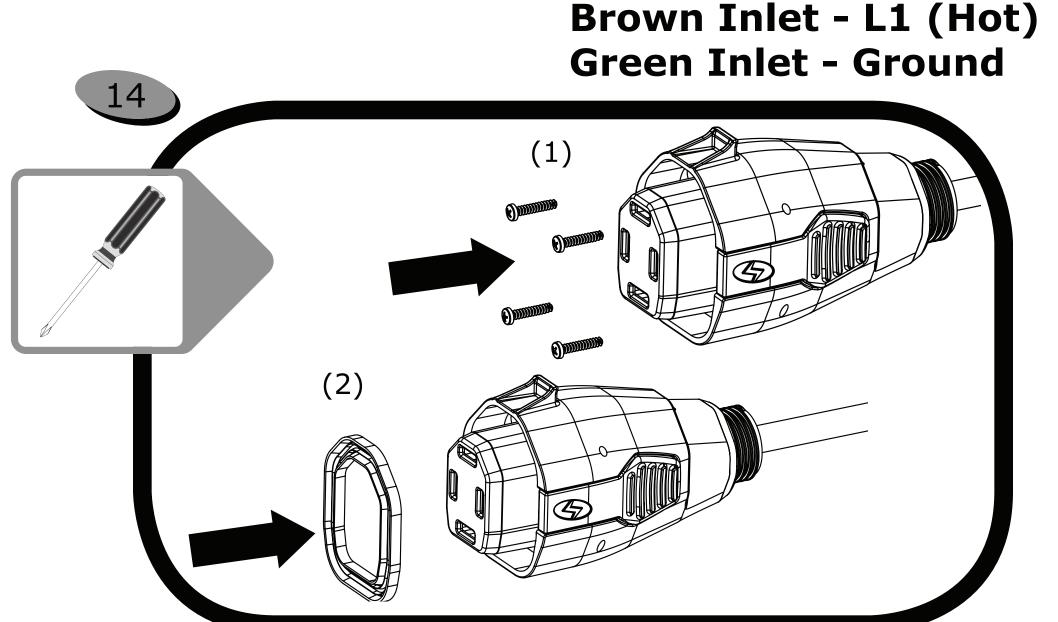
(1)Locate and install (4) #6x1" screws (included) into corresponding inlet holes as shown. Use Philip's #2 and carefully screw components together by hand only. Do not over tighten. Max torque is: 14-20 lbs/in.
