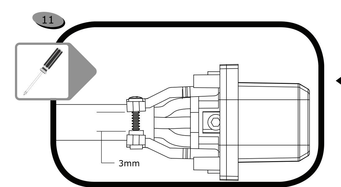
Use Phillips #2 screwdriver and tighten screws evenly about 1 turn each while alternating from one screw to the other until cable is sufficiently captured. Do not exceed 14lbs/in torque specification. Do not over tighten screws into cable clamp swing arm. A small gap as shown is acceptable, and should be even on both sides. About a 3mm gap is correct. No gap may occur for smaller diameter cords.
