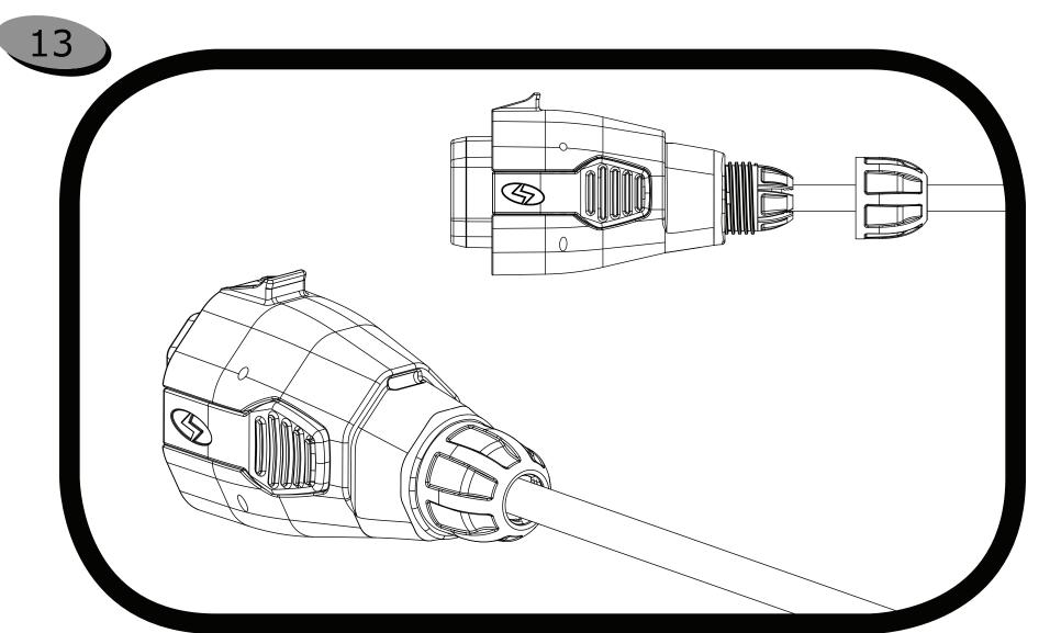
Carefully push grommet into crimp. Push grommet and crimp into threaded adapter. Slide strain relief over crimp grommet and thread onto adapter.
