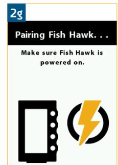
**NOTICE:** Once the downrigger is paired to the Fish Hawk, both need to be powered on in order for them to communicate. If you wish to remove the Fish Hawk to rebuild the network, or assign a new Master downrigger, you must clear the network on the downrigger and re-pair the Fish Hawk with the new Master downrigger.
