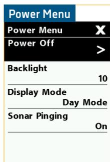
**NOTICE:** When the downrigger is connected to a Network with other downriggers, a Power Off All option is available in the Power Menu. This allows all of the downriggers to be powered "off" at once.
