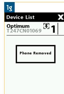
**NOTICE:** Forgetting the phone, Humminbird, Fish Hawk or downrigger removes them from the network. The Cannon app will not work until you pair the device with the Cannon app to the Bluetooth Master downrigger.
