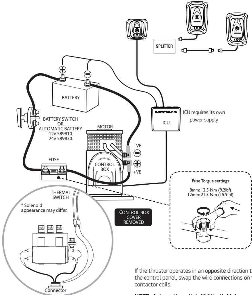
If the thruster operates in an opposite direction to the control panel, swap the wire connections on the contactor coils.
