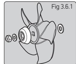
**Note: Tighten each bolt alternately a number of times to full torque.**
