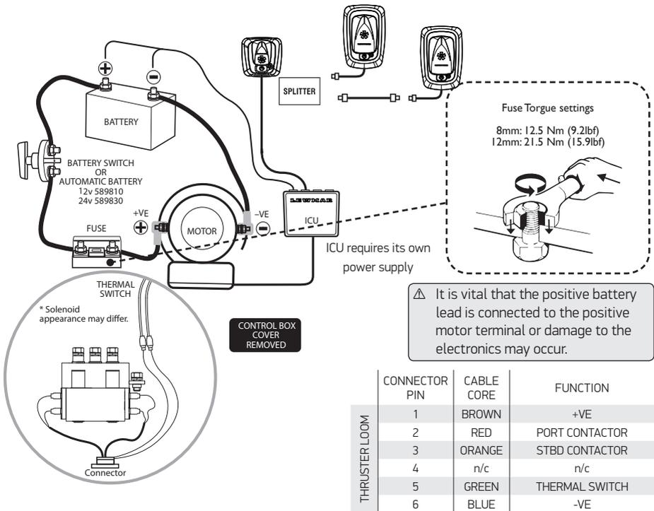
**4.2 Typical electrical layout model 250TT & 300TT**
