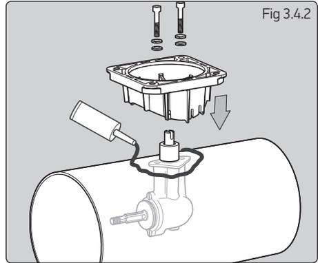
**NOTE:** Poor exterior tunnel surface could cause leakage and noise. Apply sealant to this area as required (Fig. 3.4.2).
