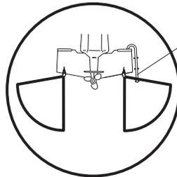
**Down Imaging®** - The starboard transducer also includes a Down Imaging beam element.
