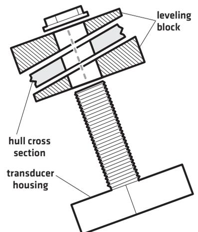
**BRONZE THRU-HULL SIDE IMAGING® TRANSDUCERS**
