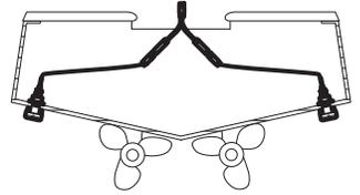
**NOTE:** A separately-purchased fairing block can also be used to create a hydrodynamic waterflow around the transducer body. The design and fabrication of this block varies greatly with different hull shapes; therefore, it should be customized by a qualified marine technician. If you plan to install a fairing block, the transducer must be mounted at 20 degrees.
