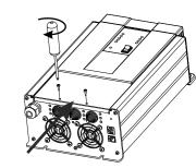
When all connections are made and double checked, slide the red connection compartment cover to it's original position again and relocate the two screws.
