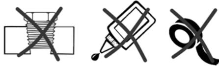
Use only bonded rubber/metal washers to seal the fittings.
