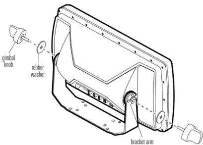
**NOTE:** If you prefer to mount the control head overhead, flip the bracket to the top of the control head. The opening in the gimbal bracket arms must face the rear of the control head.
