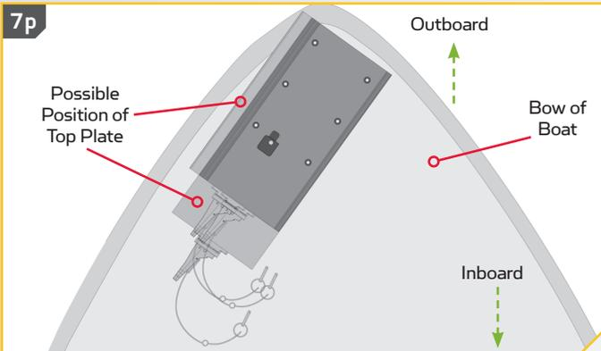
**NOTE:** Make sure that the motor will not encounter any obstructions when sliding the motor on and off the quick release bracket. The exact placement of the motor and Electric Steer Quick Release Bracket when mounting may vary depending on the boat, boat deck, and which base extrusion or bracket the quick release bracket is being mounted to. The Ultrera motor cannot be deployed before mounting and connecting a power source.
