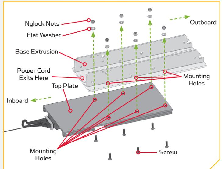
**NOTE:** If you are mounting an Ultrera to the Electric Steer Quick Release Bracket, the Clipped Washers that were previously used to install the motor to the boat, or included in the mounting hardware that came with the Ultrera motor should be used. Place the Clipped Washer above the Base Extrusion, between the Base Extrusion and the Nylock Nut. Refer to the Ultrera Owner's Manual online at [minnkotamotors.com](http://minnkotamotors.com) for complete details on mounting the Ultrera.
