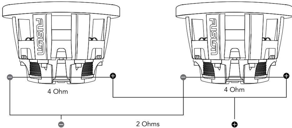
$$\frac{R1 \times R2}{R1 + R2} = \text{LOAD IMPEDANCE}$$
