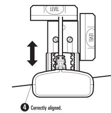
**Downward Slant:** The transducer has a natural downward slant of 4 to 5 degrees from leading edge to trailing edge. Looking at the back of the transducer, the seam should be slightly below the bottom of the
