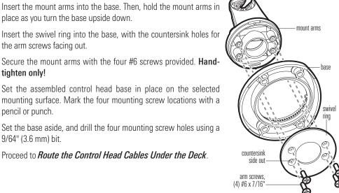
Tilt and Swivel Mount Control Head Base Assembly
