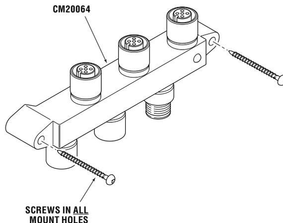
Figure 3-7. Alternative CAN2 6-port hub connection (available separately).
