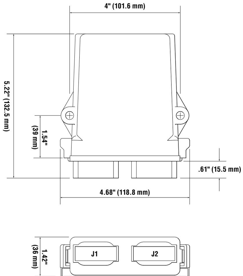
Figure A-4. Single Lever Interface – Mounting dimensions. NOT A TEMPLATE.
