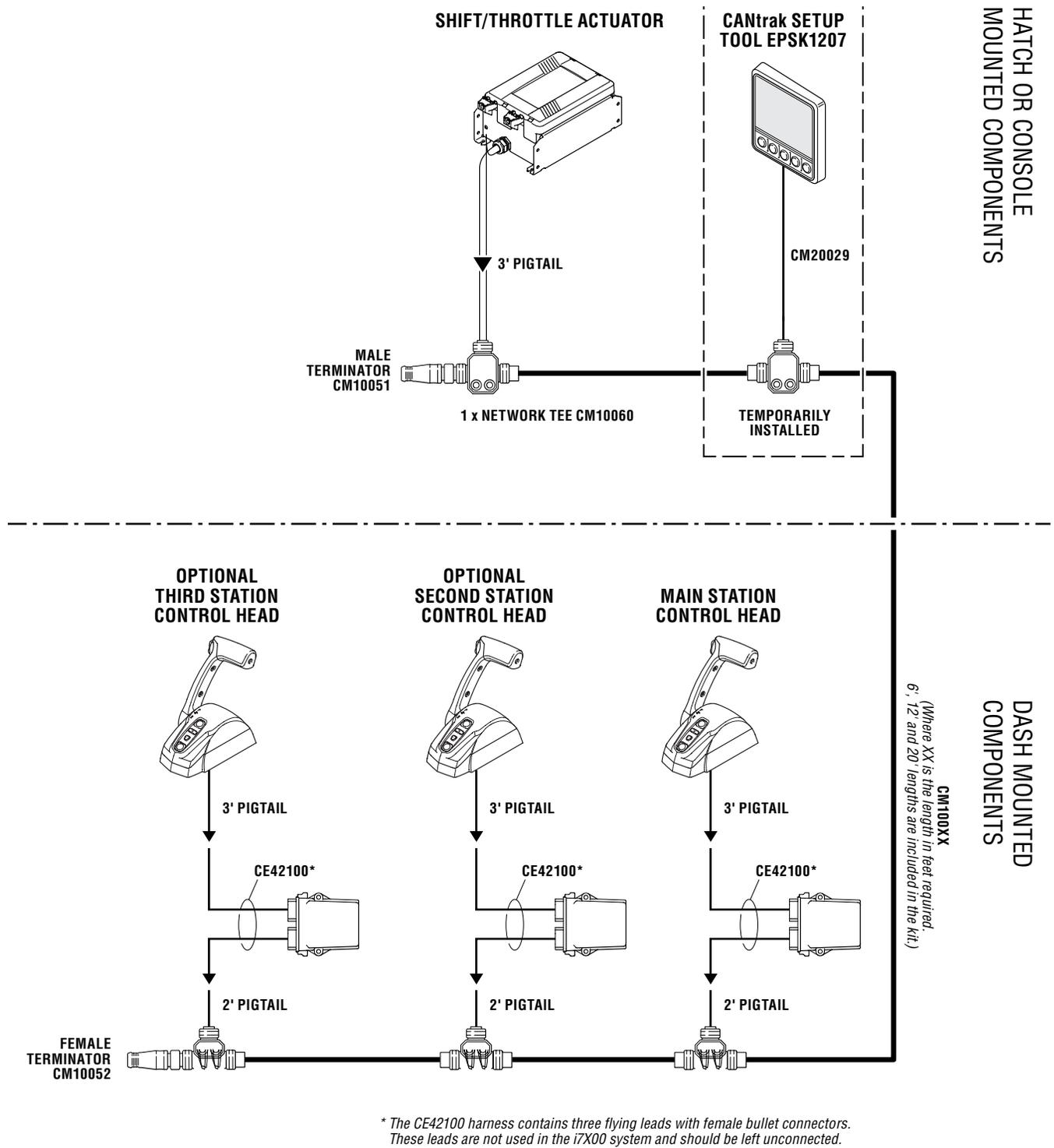
Figure 3-5. CAN2 wiring diagram, triple station, single engine.
