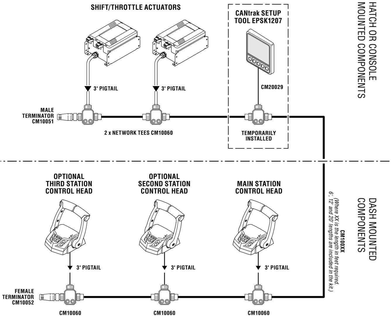
Figure 3-4. CAN2 wiring diagram, triple station, twin engine.
