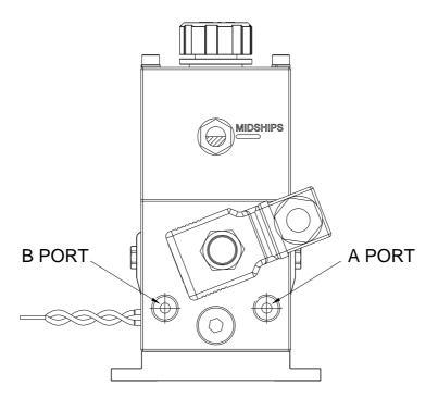
Adaptors are available to convert the ports to SAE, NPTF or Metric threads.
