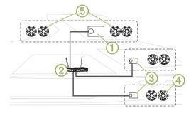
In the image above, one Apollo RA670 stereo ① connects to a wireless router ② and to two Apollo SRX400 zone stereos ③.
