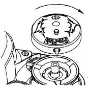
5. Lightly grease the exposed end of the Main Shaft, making sure you do not get grease in the threaded hole in the end of the shaft. Place Pro-fish Cap assembly onto the Shaft and screw down by hand.
