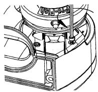
7. Undo & remove Stripper Screws using allen key provided.
