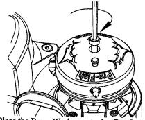
6. Place the Brass Washer onto the Cap Screw. Put Loctite (provided) onto thread of bolt and fit into the end of the Main Shaft. Tighten up using allen key provided (21Nm, 15.4 lbf/ft). Allow at least 15mins for Loctite to cure before use.
