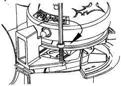
9. Fix Stripper & Cam into place using two new longer screws supplied. Use Loctite on the threads of the screws prior to fitting them. Allow at least 15mins for Loctite to cure before use.
