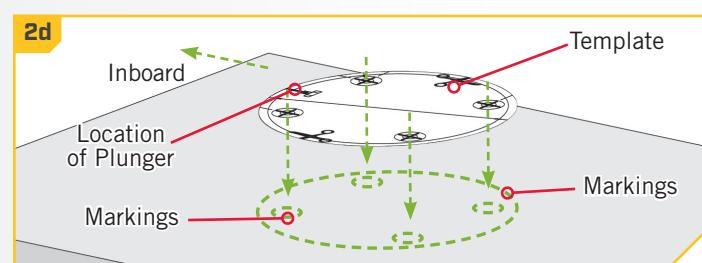
**NOTICE:** Drill the holes for the screws completely through to prevent splitting the boat deck.
