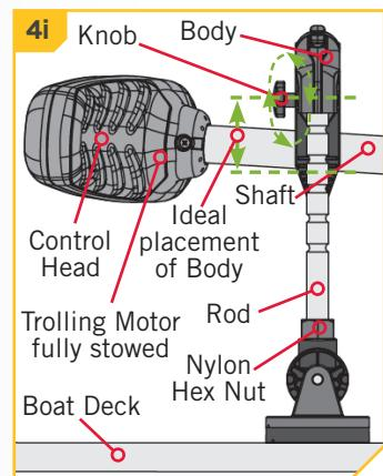
**NOTICE:** When cutting the Rod at least one notch on the Rod must remain. If unsure, leave the Rod longer, and cut off fewer notches and test after each notch is removed before finishing the installation, or have the bracket installed by a qualified marine installer.
