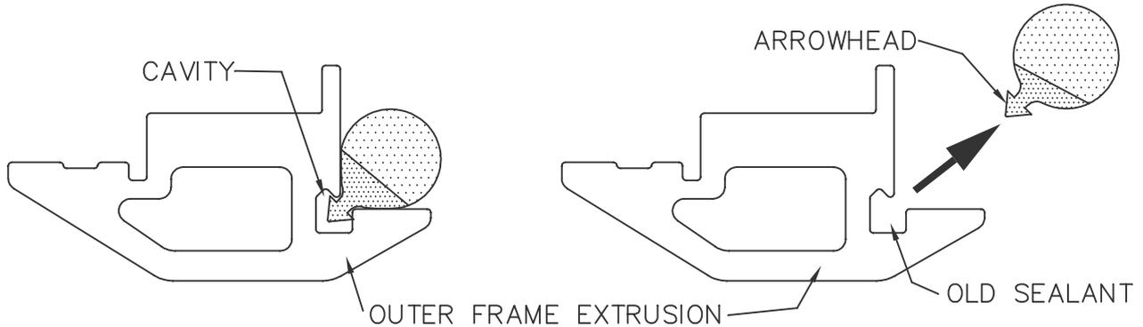
WHEN REFITTING THE SEAL IT IS IMPORTANT TO NOTE THAT THE SEAL IS NOT THE SAME ON BOTH SIDES, THERE IS A SLIGHT STEP WHICH APPEARS AS A LINE ALONG THE SEAL. ON ONE SIDE OF THE SEAL THE STEP IS FURTHER AWAY FROM ONE SIDE THAN THE OTHER. FIT THE SEAL WITH THE STEP FURTHEST FROM THE ARROWHEAD CLOSEST TO THE CENTRE OF THE PORTLIGHT.
