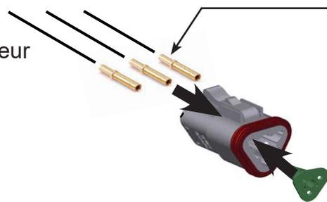
**Crimp Terminal on Wire, then insert thru connector.**
