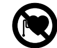
Persons with cardiac pacemakers or other medical implants must maintain a distance of 50 cm to the system.
