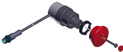
Fig. 46: Emergency Off switch installation drawing
