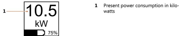
Fig. 63: Power consumption display view
