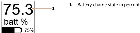
Fig. 62: Battery charge state display view
