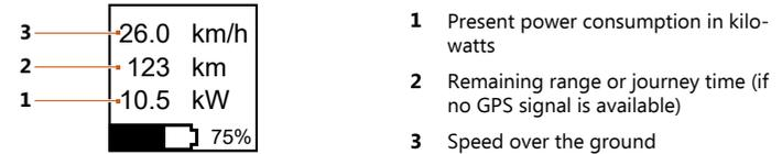
Fig. 65: Speed, range and power consumption display view
