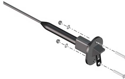
Fig. 51: Kill switch exploded drawing
