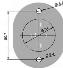
Fig. 50: Kill switch installation drawing
