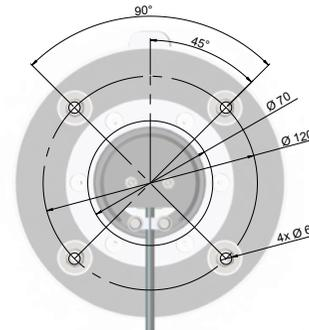
Fig. 46: Remote throttle installation drawing
