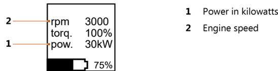
Fig. 64: Engine speed, torque and power display view
