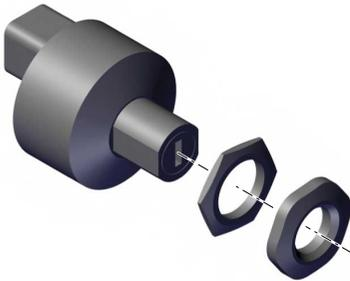
Fig. 53: Key switch exploded drawing
