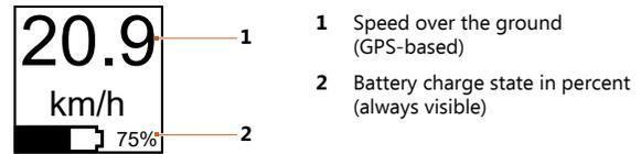
Fig. 60: Speed display view
