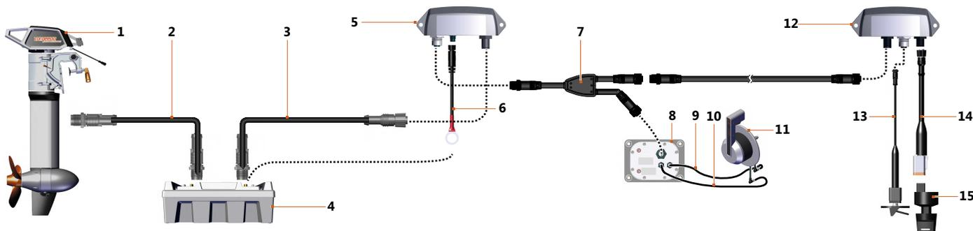
Fig. 54: Cabling of the remote throttle unit
