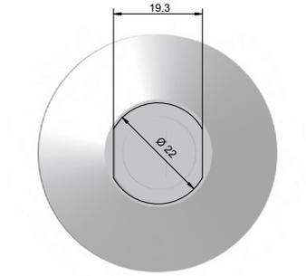
Fig. 52: Key switch installation drawing
