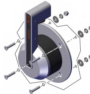
Fig. 47: Remote throttle exploded drawing
