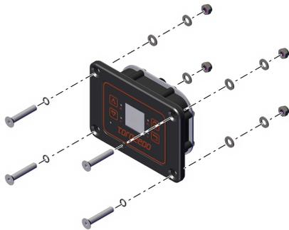
Fig. 48: Display exploded drawing
