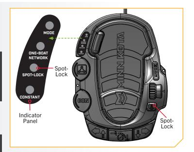
**NOTICE:** Pressing any button on the Foot Pedal or manually steering the motor with the Foot Pedal will disengage Spot-Lock. Manually steering or adjusting the Prop Speed with a paired remote will also cancel Spot-Lock.
