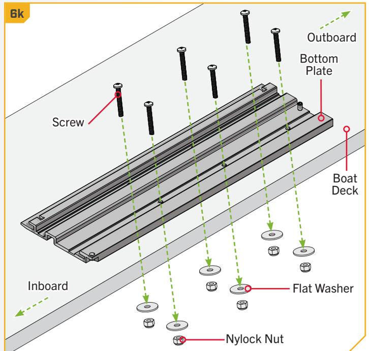
**NOTICE:** The mounting surface for the Bottom Plate must be completely flat; otherwise, the Top Plate will not fit correctly. Rubber washers can be used to shim the Bottom Plate flat before the hardware is tightened.
