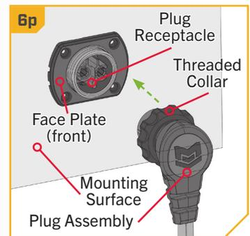
**NOTICE:** Use the Dust Cap when the plug is not in use to insure optimal water-tight protection to electrical contacts.
