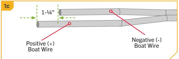
**NOTICE:** The ends of the Boat Wires may have any sort of electrical connector that should be removed.
