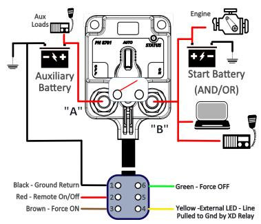
A) 88xx-xxxx Part Numbers Use a DTM 06-6S Connector End. Customer Supplies DTM04-6P or Cuts & Uses Individual Wire Terminations.
