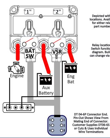
Depicted with manual override knobs in all locations. Availability of manual override knob for either relay position determined by the part number. See part number guide for further details.
