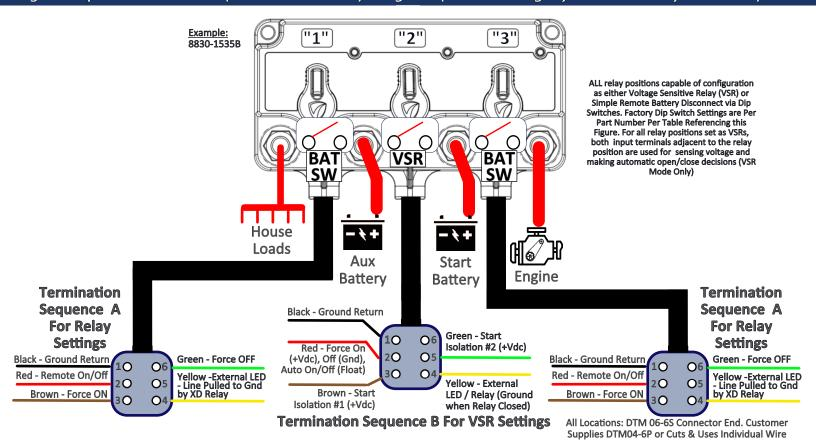
Fig 8 - Triple XD - 87 Series (Connection Diagram)
