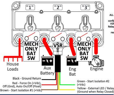
ALL switch positions capable of configuration as either VSR/ACR or Simple Relay via Dip Switches. Control wire responses change accordingly
