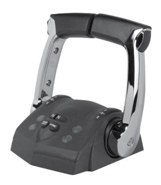
Figure 3-1. i7700 Dual Lever Control Head.
