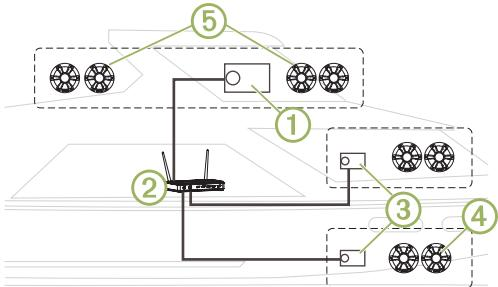
In the image above, one Apollo RA770 stereo ① connects to a wireless router ② and to two Apollo SRX400 zone stereos ③. The two FUSION PartyBus stereo zone stereos can stream sources from the FUSION PartyBus stereo.
