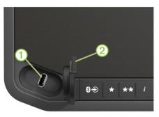
① USB port for your mobile device connection or a low-profile USB flash drive. Charges your mobile device.
