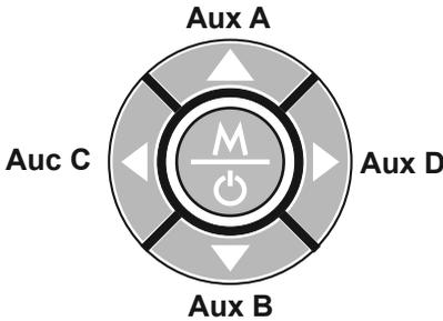
Example set up is for a windlass plus auxiliary equipment such as a cleat, using a single AA702 base station.
