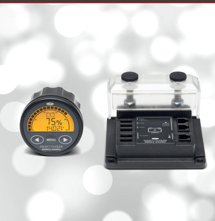
Complete battery status information at a glance (%, V, A, Ah, W, h:m, °C) Supports up to three battery banks (12V, 24V and 48V) Very simple 'Plug and Play' installation Perfect integration with TBS DC Modular products
