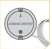
**NOTE:** If replacement screws must be used, ensure that they are high grade non-magnetic stainless steel.
