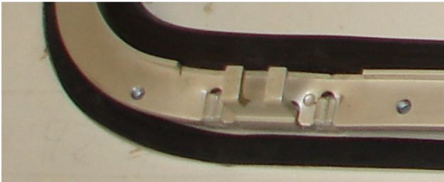
Handle catch fitted with pressed / staking process
