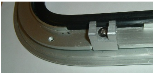
Handle catch fitted with screw
