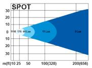
Peak Beam Intensity: 110,000 Candela Maximum Beam Distance: 683m/2240 ft. Beam Angle: 10° Spot
