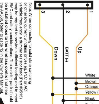
**IMPORTANT:** All windlass controls must be wired in parallel
