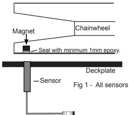
**Note:** If it is not possible to align the sensor and magnet exactly the AA grey sensor may be fitted up to 20mm out of alignment. The AA black sensor and the reed switch sensor must be directly aligned.
