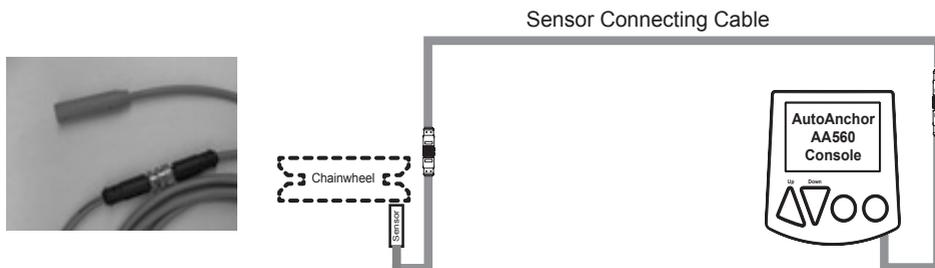
The sensor cable and the console sensor cable are fitted with female plugs. Sensor connecting cable with a male plug at each end is available in the following lengths:
