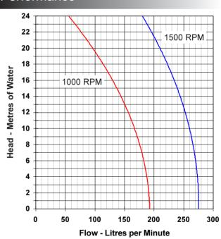
**Note**: Performance shown is for a new pump, fitted with a Neoprene impeller, pumping water at 20°C, performance may vary by up to 15%. Consult factory for performance of alternative impeller compounds.
