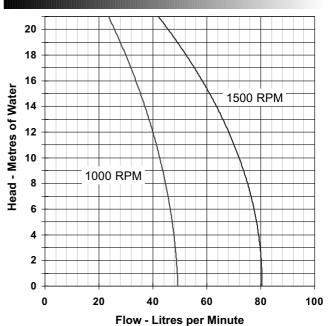
Note: Performance shown is for a new pump, fitted with a Neoprene impeller, pumping water at 20°C, performance may vary by up to 15%. Consult factory for performance of alternative impeller compounds.
