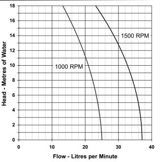
**Note** : Performance shown is for a new pump, fitted with a standard pressure Neoprene impeller, pumping water at 20°C, performance may vary by up to 15%. Consult factory for performance of alternative impeller compounds.
