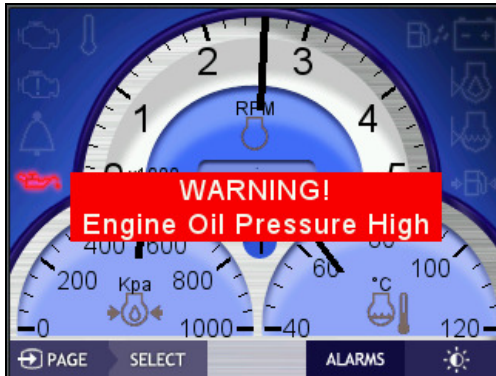
Figure 46: EGM Performance Alarm and Warning
